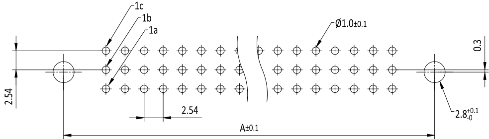
RECOMMENDED PCB LAYOUT(TOP VIEW) TOLERANCES: ±0.05mm
