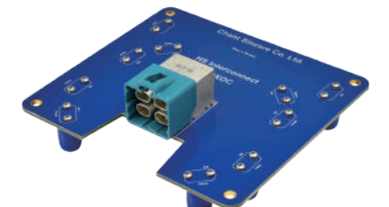
70244030010 CAR EtherNet Plug 2x2 R/A Type Coding:A,B,C,D,E,F,G,H,J,K,L,M,O,Z Positions:04
