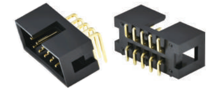
514 Box Header / Box Header SMT Pitch:2.54mm Positions:10,14,16,20,24,26,30,34,40,50,60,64
