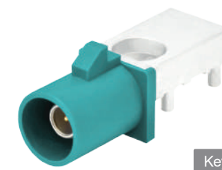
541 FAKRA Plug R/A Middle Type, CH=0.24 Coding:A,B,C,D,E,F,G,H,I,K,L,M,N,Z Positions:01
