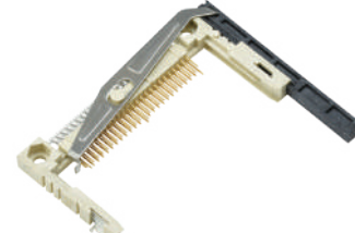
575 Compact Flash Card Socket Type II Slim Type Positions:50
