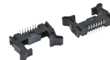
521 Ejector Header SMT Pitch:2.0mm Positions:6~64
